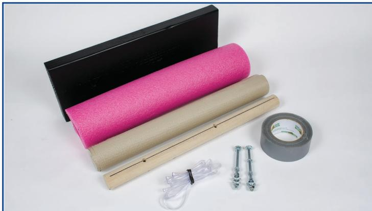
All of the materials you need can be easily found. The simulated limb is constructed using a foam pool "noodle" as the main structure of soft tissue, a wooden dowel rod as a long bone in the center of the foam noodle, and an outer covering of shelf liner skin. A length of tubing is also run through the center of the foam to simulate a deep lying blood vessel. The constructed limb is connected to a solid wooden base using carriage bolts.
