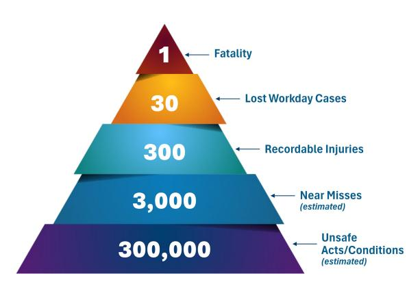
The consequences of safety incidents range from unsafe acts and near misses to serious injuries and fatalities. The number of incidents compared to their seriousness can be represented as a pyramid. The safety pyramid is also referred to as the accident pyramid, Heinrich's triangle, or Bird's triangle.
